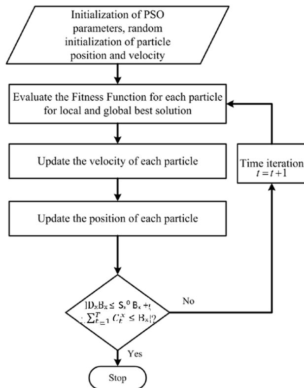
Fig: 2. Flow chart for PSO for phase balancing
