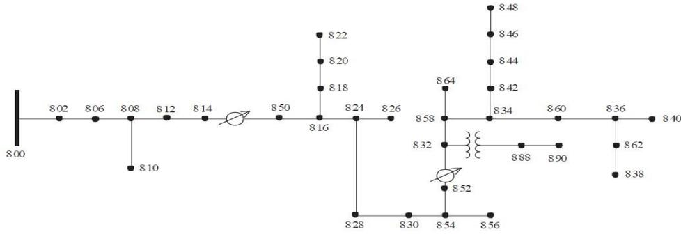
Fig: 3. IEEE 34 bus test feeder
