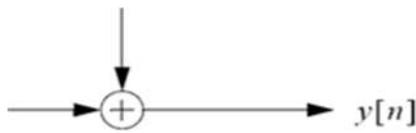
Fig 6 Adder block in FIR
