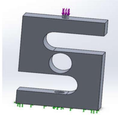
**Figure 05: Applied force and Boundary Conditions**
