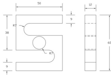
Figure 01. 2d model of transducer
