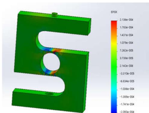
**Figure 07. Strain distribution**
