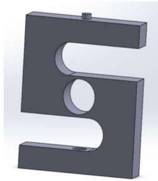
**Figure 02. 3D model of a load cell element**
