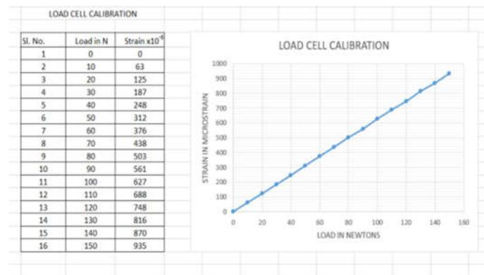
**Figure 10. Calibration curve for sensor**
