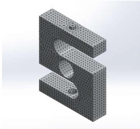
Figure 03. Finite mesh element of a Load Cell
