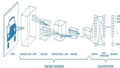
Fig. Convolutional Neural Network (CNN)
